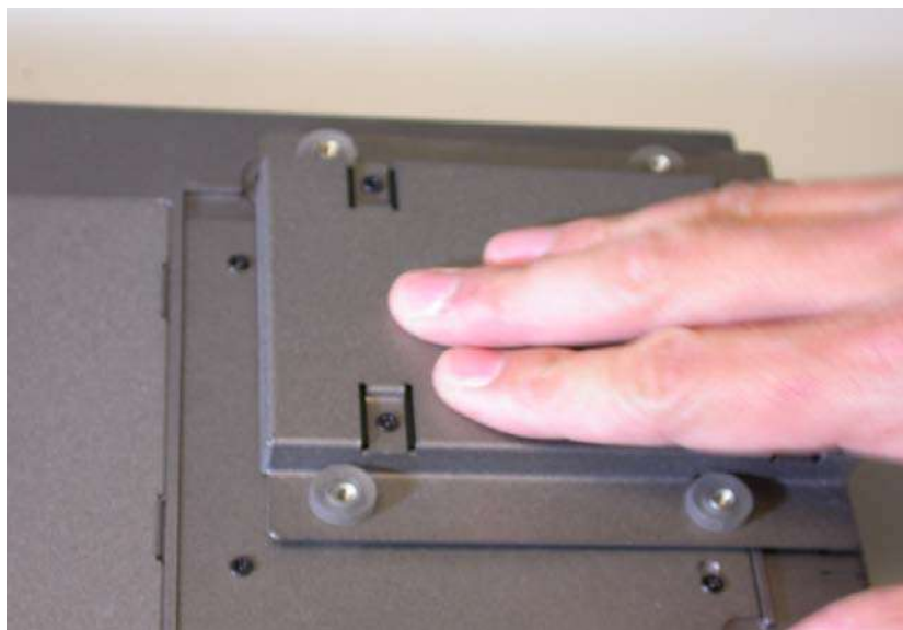
Figure E.12: Placing the HDD holder - 2
