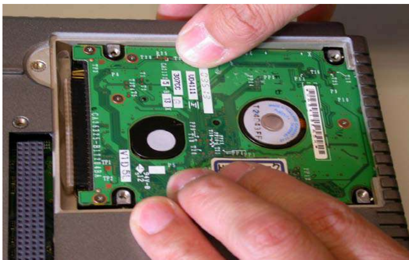
Figure E.18: Inserting the HDD
