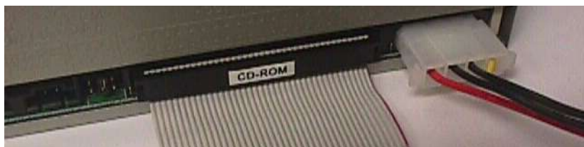
Figure D.7: Plugging in the CD-ROM Drive
