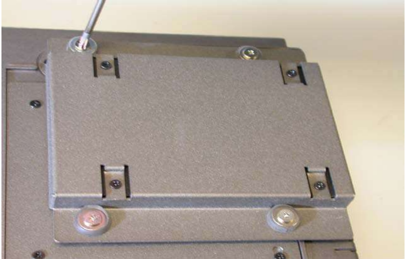
Figure E.13: Fastening the HDD holder
