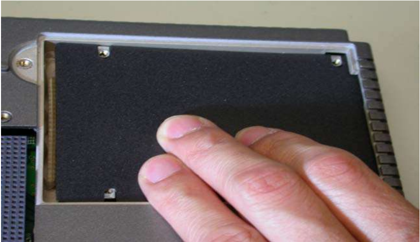
Figure E.19: Laying in the HDD insulator
