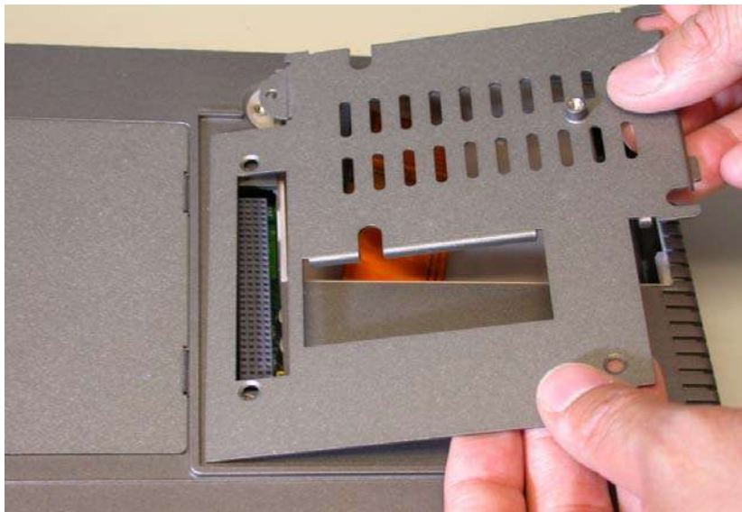
Figure E.1: Removing the HDD cover
