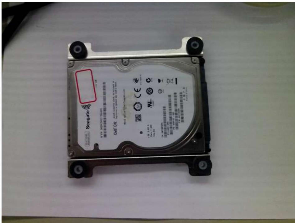
Figure C.3 Installing HDD in the holder
