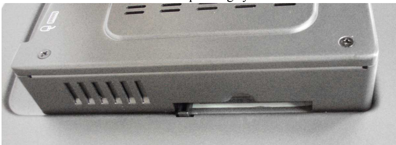
Figure 2.2: Install CompactFlash Memory Card
