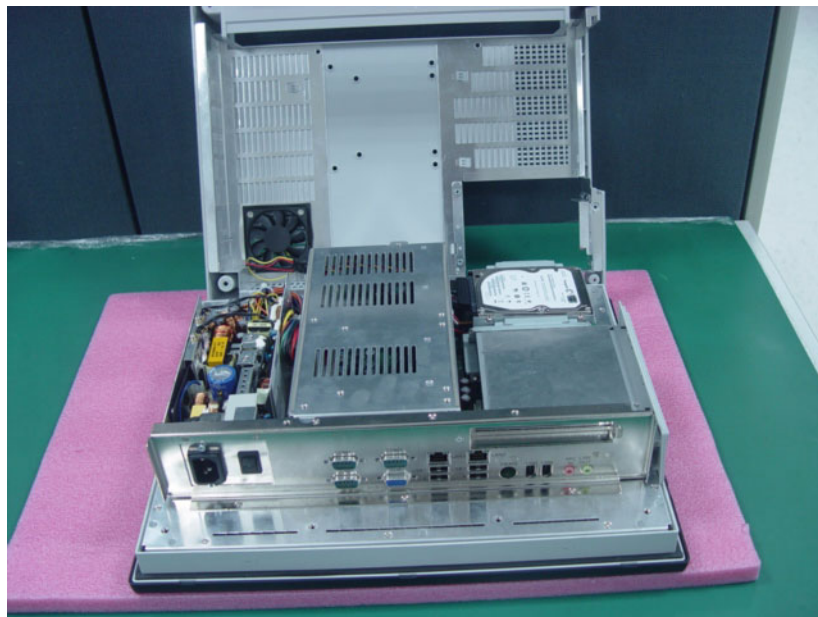
Figure 4.1 Unfastening the Rear Cover
