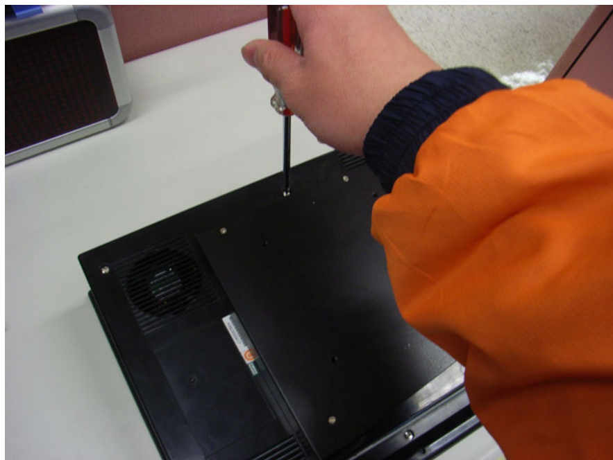
Figure 4.1 Unfastening the Rear Cover
