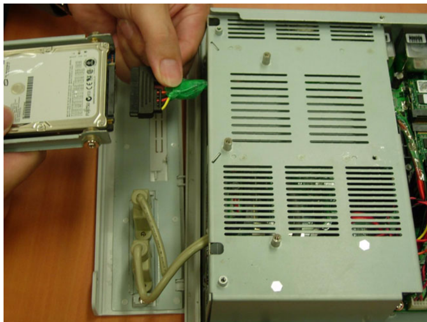
Figure 4.7 Plugging in the SATA Cable
