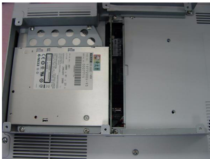
Figure 4.16 Riser Card and ODD Connection
