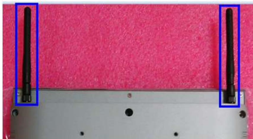
Figure 2.21 Location of external antennae
