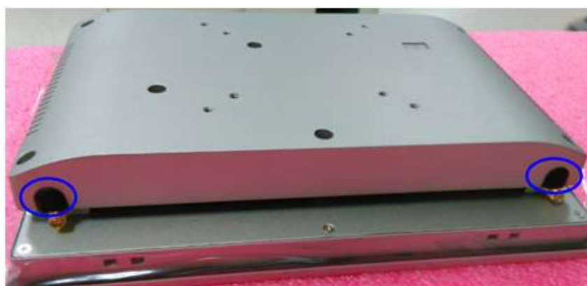
Figure 2.19 Removing plugs for the antennae
