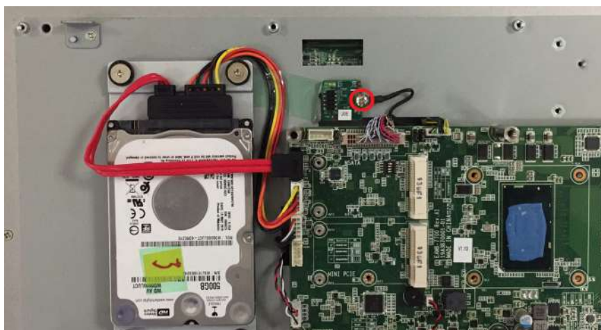
Figure 2.18 Fix TPM card with LVDS cable
