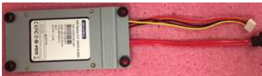
Figure 2.10 Secure SATA HDD with screws
