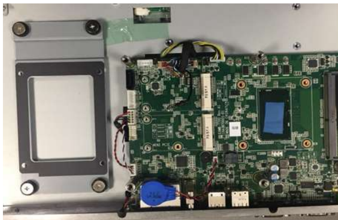
Figure 2.7 Retention screws on HDD bracket
