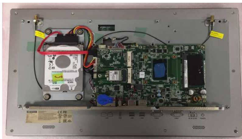
Figure 2.15 Full-size mini PCIe LAN antenna cables
