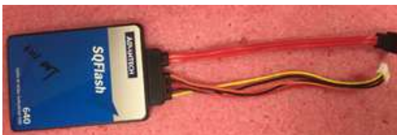
Figure 2.9 SATA cable connected to SATA HDD
