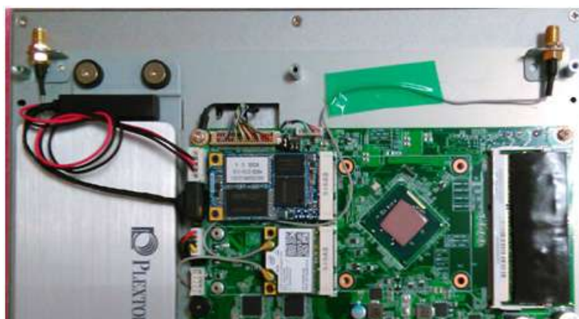
Figure 2.18 Half-size mini PCIe LAN antenna cables
