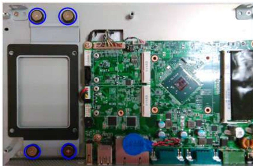
Figure 2.8 Retention screws on HDD bracket
