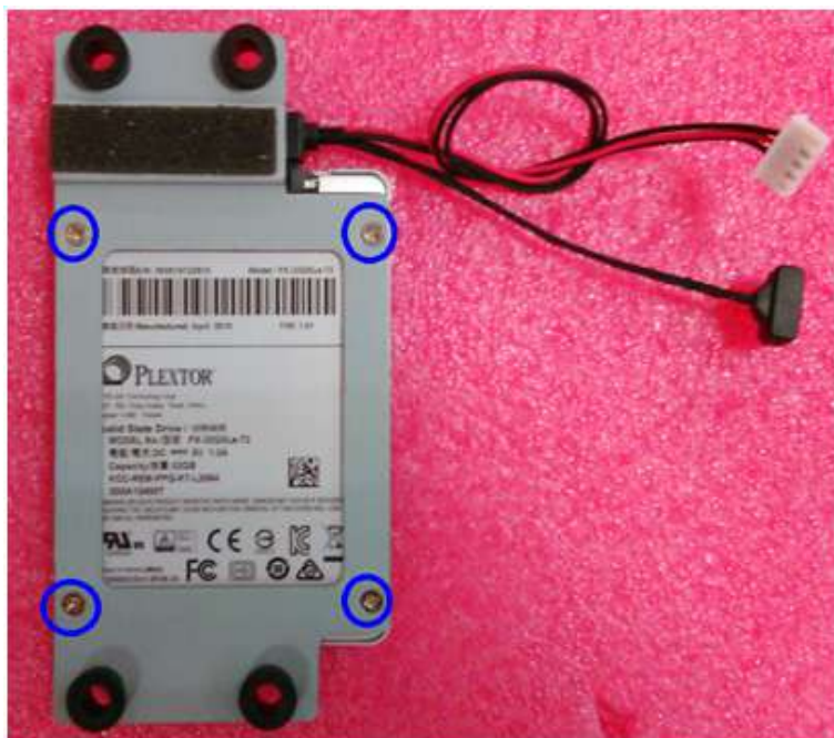
Figure 2.11 Secure SATA HDD with screws
