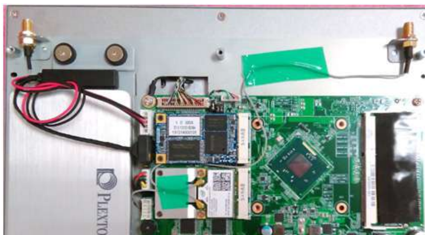
Figure 2.17 Full-size mini PCIe LAN antenna cables
