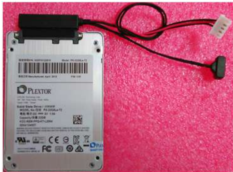
Figure 2.10 SATA cable connected to SATA HDD
