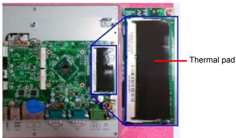
Figure 2.7 Thermal pad placed on the memory card
