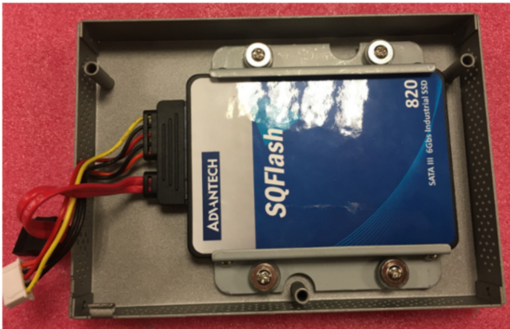
Figure 2.10 Installing the HDD into the HDD cover
