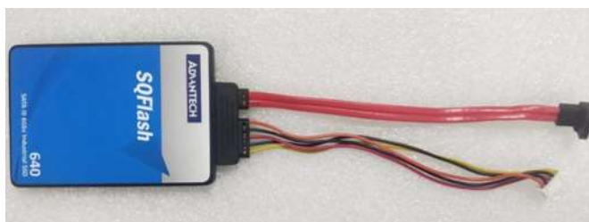
Figure 2.9 SATA Cable Connected to the SATA HDD
