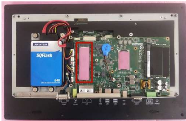
Figure 2.13 Affix the Thermal Pad to the M.2
