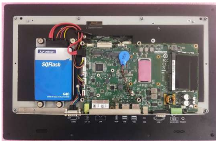
Figure 2.11 SATA HDD Connected to the Motherboard
