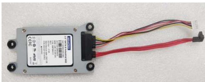
Figure 2.10 Secure the SATA HDD with Screws
