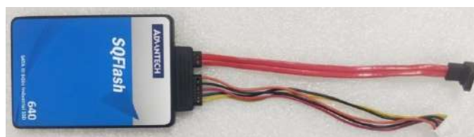
Figure 2.7 SATA Cable Connected to SATA HDD
