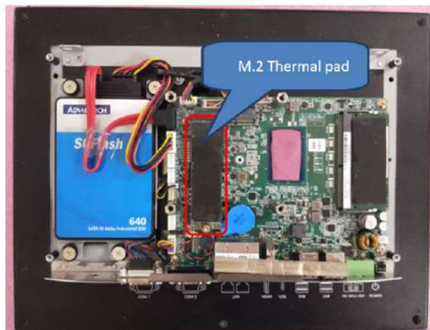
Figure 2.11 Apply the Thermal Pad to the M.2
