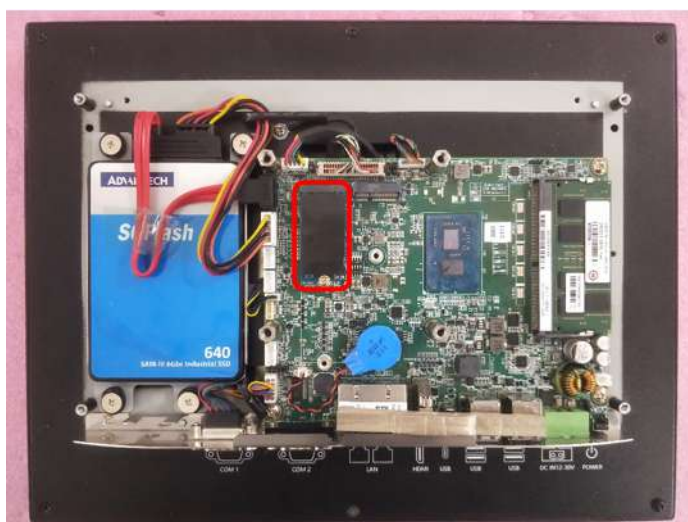
Figure 2.14 Apply the Thermal Pad on the M.2 2242 Card
