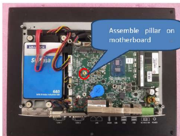
Figure 2.12 Install the Pillar on the Motherboard
