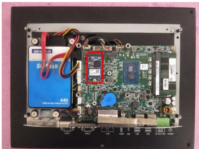
Figure 2.13 Install the M.2 2242 Card on the Motherboard
