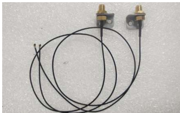
Figure 2.15 Assemble the Bracket with the Antenna Cable
