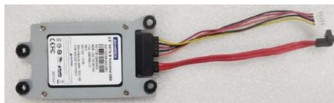
Figure 2.8 Secure SATA HDD with Screws
