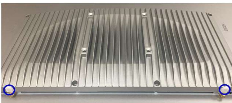
Figure 2.16 Removing plugs for the antennae
