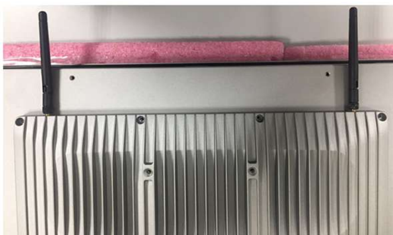
Figure 2.17 Location of external antennae
