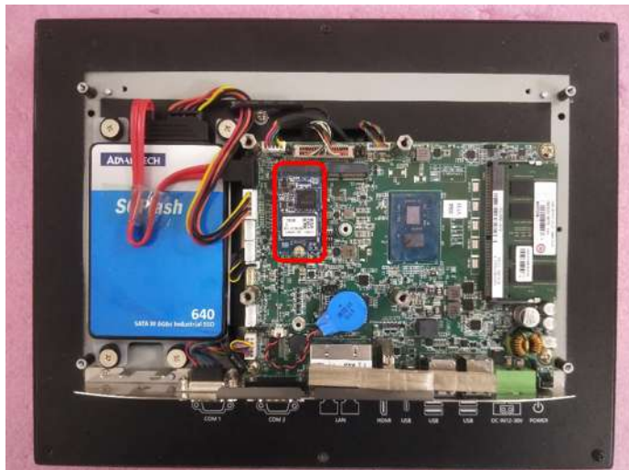
Figure 2.13 Install the M.2 2242 Card on the Motherboard
