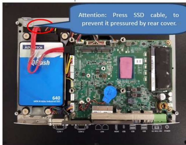
Figure 2.9 SATA HDD Connected to the Mainboard
