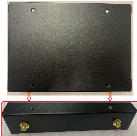
Figure 2.5 Antenna cable assemble on rear cover
