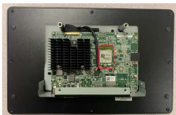
Figure 2.4 Installing the wireless LAN card
