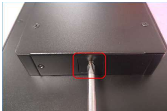
Figure 2.1 Remove SD card bracket
