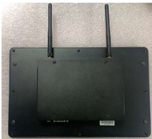
Figure 2.7 Location of external antenna
