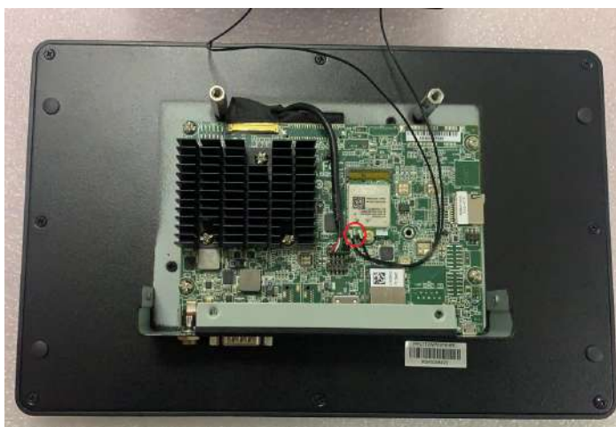
Figure 2.6 Connect antenna cable with wireless LAN card
