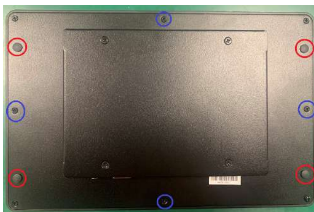
Figure 2.18 Remove rear cover
