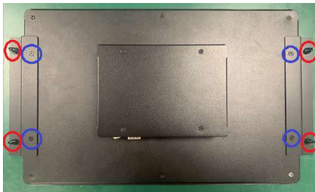
Figure 2.20 Install panel mount bracket
