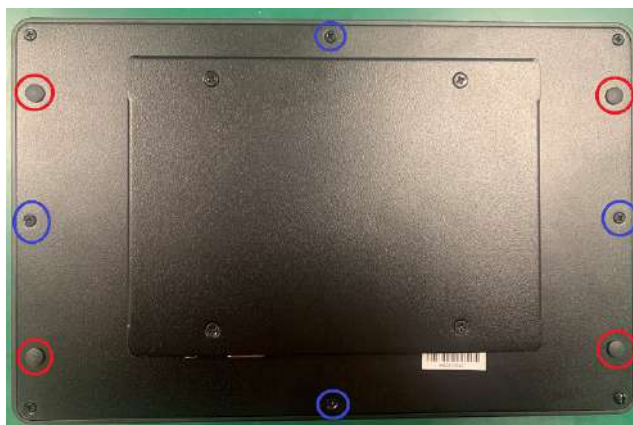
Figure 2.12 Remove rear cover
