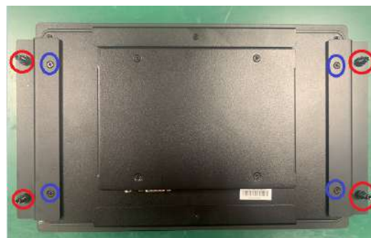
Figure 2.14 Install panel mount bracket
