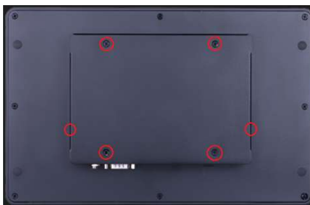
Figure 2.3 Retention screws on rear cover
