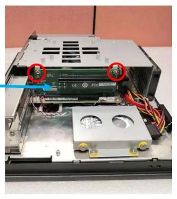
3. Install the graphic card into the PCIe slot and lock the screws
