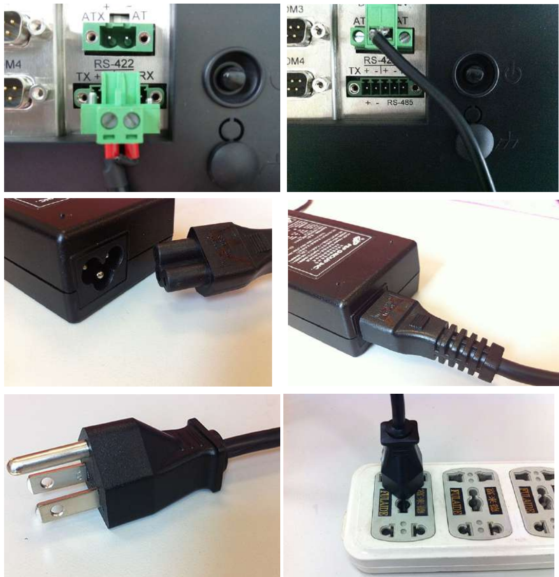
Figure 2.4 Connecting the Power Cable
