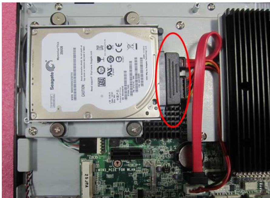
Figure 2.12 Plugging HDD Wire
