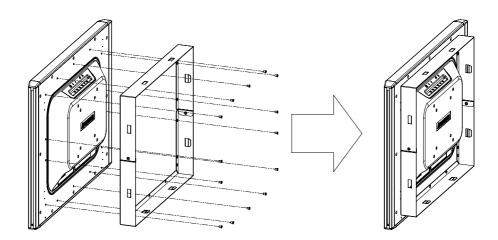
2. Then attaching 8 panel mount clamps, which are also included in the accessory box, to the brackets for fixing ITM-5117.
