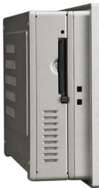
Figure 2.2 Install CFast Memory Card
