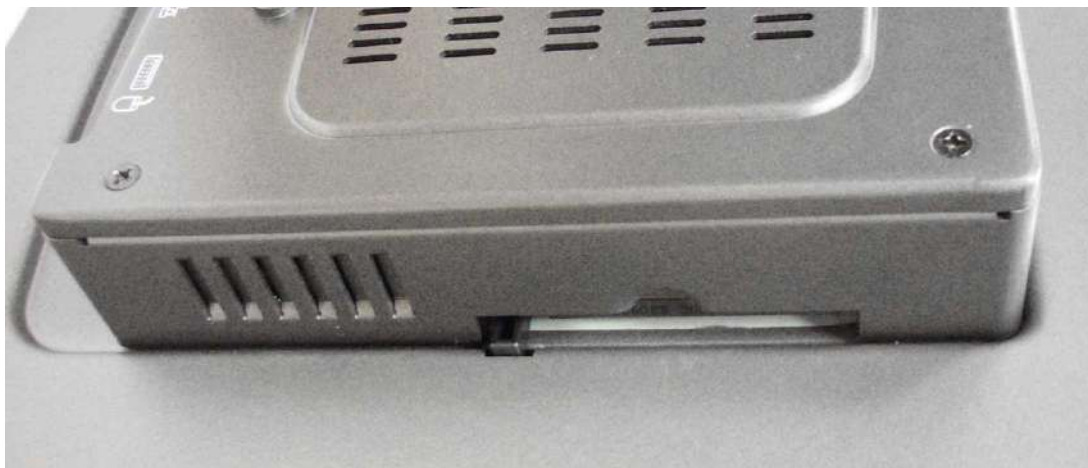
Figure 2.2 Install CFast Memory Card
