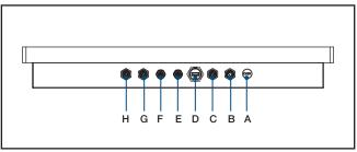
A. Exhaust Valve E. LAN 1 F. LAN 2 B. Power Connector C. USB 2.0 x 2 G. COM 1 D. USB 3.0 x 1 H. COM 2
