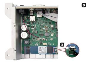
Secure the M.2 NVMe/SATA SSD with the screw which is unscrewed in the first step.
