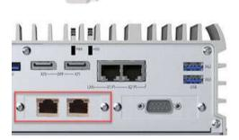
Secure the additional interface-card in the position of the COM interface with screws.
