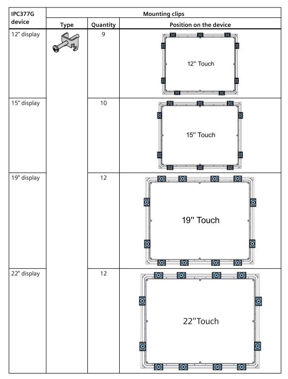
The following table shows the type, number, and position of the mounting clips needed for the respective devices.
