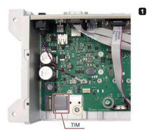
To install M.2 NVMe/SATA SSD with form factor 2280, remove the screw M3x4 marked in red.
