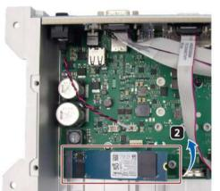
Align the golden finger on the M.2 NVMe/SATA SSD to the motherboard, then press firmly until the M.2 NVMe/SATA SSD is completely seated on the slot.
