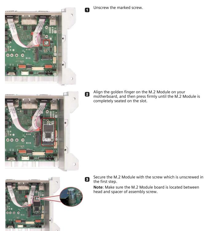
If the M.2 Module has a cable with an additional interface-card connected to the housing opening, you need to do the following procedures:
