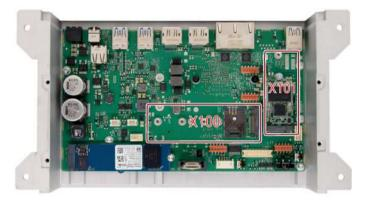
Siemens IPCs provide the standardized openings in the housing to extend the devices with additional external interfaces.
