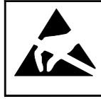
**ESDs** can be destroyed by voltage and energy levels which are far below the level perceptible to human beings. Such voltages already occur when a component or a module is touched by a person who has not been electrostatically discharged. Components which have been subjected to such overvoltages cannot, in most cases, be immediately detected as faulty; the fault occurs only after a long period in operation.
