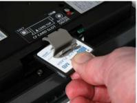
OI Touchscreens (excluding 4.6" HG1F) support Compact Flash (CF) Cards with up to 512 MB of memory. In addition to storing recipe, alarm and trending data, the CF Card can also store screen captures in a BMP format for documentation purposes. The CF Card can hold one or more projects and you can easily transfer a project directly to another touchscreen by simply inserting the card into the second touchscreen and downloading what you need.
