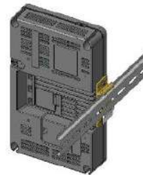
<Example of Din rail installation of the Main Unit >
