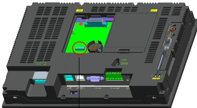
No.3 Switch (BACK UP BATTERY On) to be located toward A
