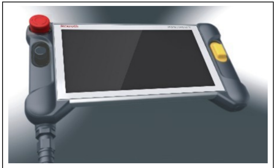
Fig. 12-1: Hand-held terminal VH2110
