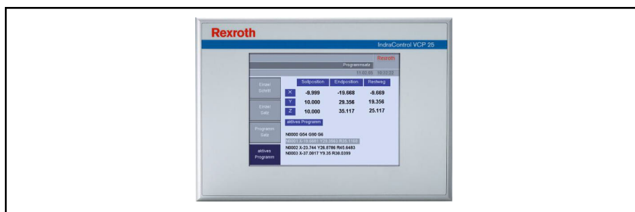
Fig. 9-5: VCP 25 small operator panel
