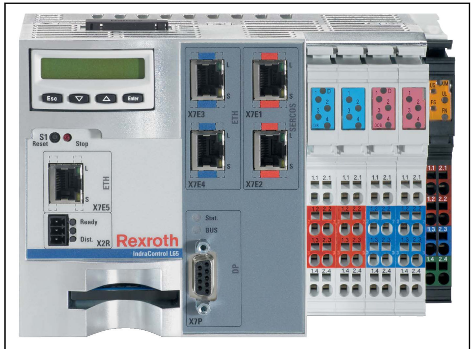
Fig. 5-1: IndraControl L65 control
