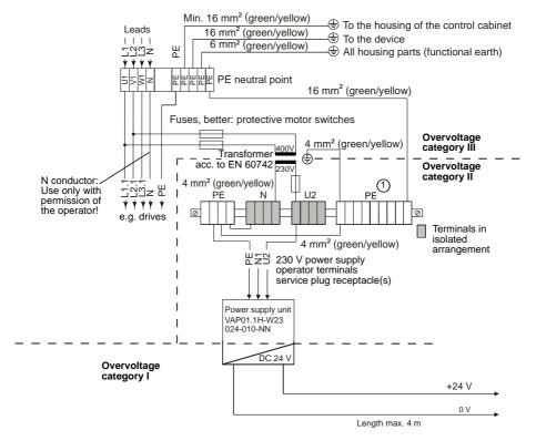
• PE bars are to be installed preferably on the mounting plate. In case of isolated PE bars, connect both ends to the mounting plate by means of copper strips with a maximum length of 20 cm. The cross-section of the copper strips has to be at least equal to that of the incoming mains cable.
