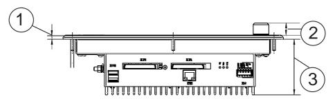
Fig. 10-2: Overview: Top view: Embedded Terminal (using the example of VEP 30.4)
