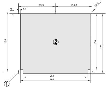
Drilled hole for the mounting bolts, bore diameter 5 mm
