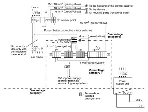
• PE bars are to be installed preferably on the mounting plate. In case of isolated PE bars, connect both ends to the mounting plate by means of copper strips with a maximum length of 20 cm. The cross-section of the copper strips has to be at least equal to that of the incoming mains cable.
