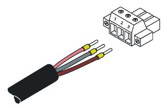
Fig. 8-4: Connecting the female connector strip
