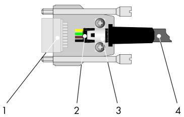
Fig. 7-37: Shielding D-SUB connectors
