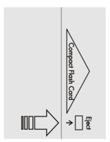
Fig. 7-36: Ejecting the memory card
