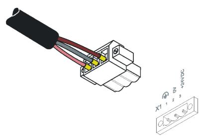
Fig. 8-5: Female connector strip is plugged on
