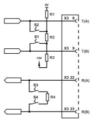
Fig. 7-8: Block diagram termination RS485
