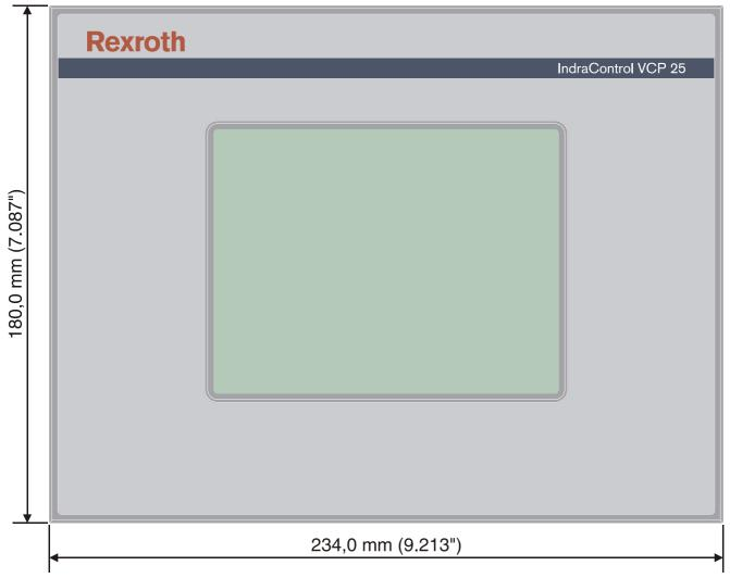
Fig. 5-1: Front panel dimensions
