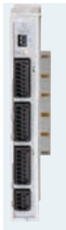
Fast I/O Function interface, high- speed inputs and outputs for short response times For implementation of I/O with very short response times; 8 inputs, 8 outputs and 8 user-configurable inputs or outputs. The inputs can be used as probes with a resolution of 1 \mu s.
