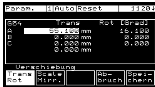
Fig. 3-10 Work offset: Translation, rotation
