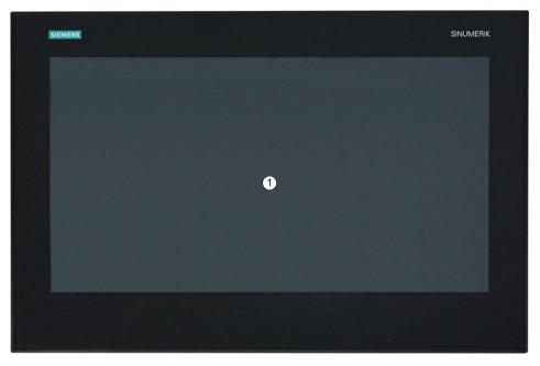
1 Multiple finger operating area for operating software (softkeys) in the display area
