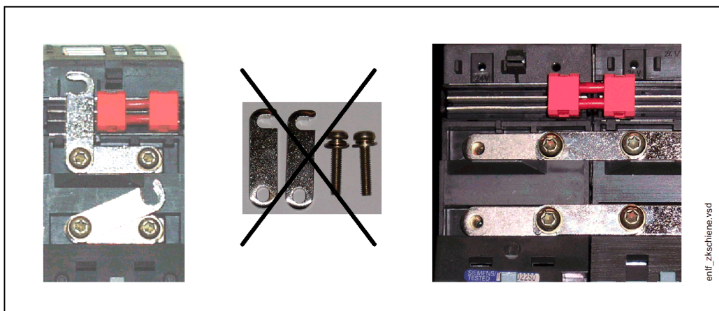
Figure 2-1 Removal of the DC link bridge
