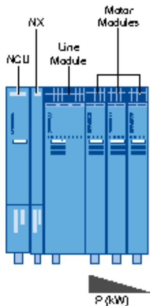
Figure 2-7 NX between NCU and Line Module
