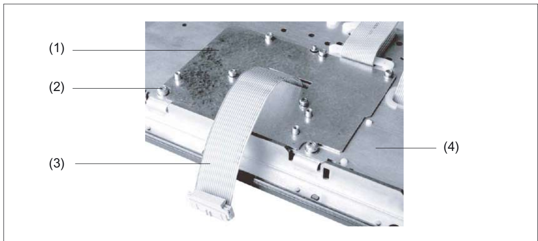
Figure 16-8 Installation of the direct control key module on the OP 012
