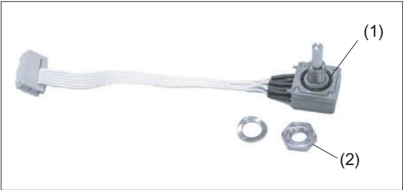
Figure 23-19 Dismantled rotary override switch
