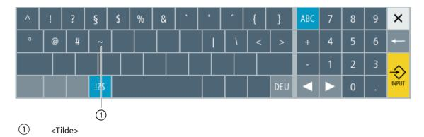
In the Editor or in alphanumeric input fields, the special character <Tilde> is entered with the <Tilde> key. In numerical input fields, the <Tilde> key changes the sign of a number between plus and minus.
