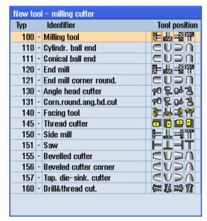
Figure 14-2 Available tools in the "New Tool - Milling Cutter" window
