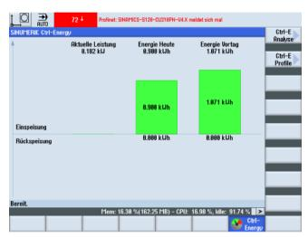
Figure 20-1 Ctrl-Energy entry screen with display of the current energy consumption
