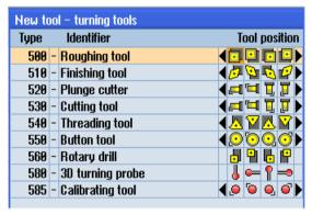
Figure 14-4 Available tools in the "New Tool - Turning Tools" window
