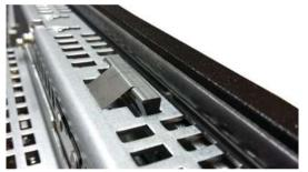
Make sure that the PPU sits firmly in the installation cutout and cannot fall out before you secure the PPU at the rear using the tension jacks.
