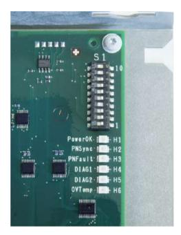
Image 4-20 Switch S1 and LEDs H1 to H6
