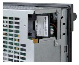
5. First, guide the metal cover at the rear into the rabbet and fix to the housing using the screw.
