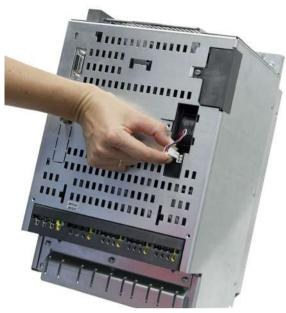
4. Remove the cable connector by gently pressing the interlock and connector together.
