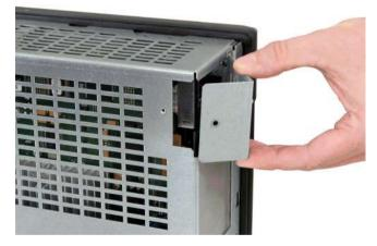
4. Attach the metal cover to the housing using the screw.
