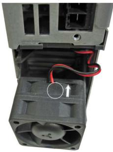
2. Insert the cable connector until it latches into place.
