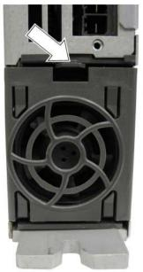
2. Remove the fan cover at the lower side of the Motor Module by releasing the snap hooks.
