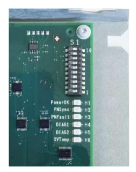
Image 4-17 Switch S1 and LEDs H1 to H6
