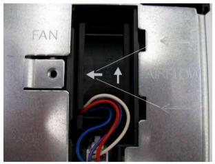
The arrows on the fan show the direction of the airflow.
