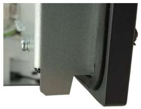
3. Tilt the PPU and press the snap mechanism to fit the device into the cutout (only for PPU 290.3)
