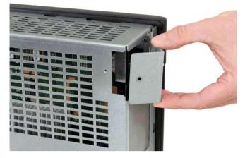
4. Remove the system CompactFlash Card from the side.
