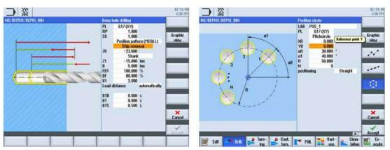
The SINUMERIK 828D offers you a unique range of CNC technology cycles for standard machining – including an engraving cycle. The assignment to the machining positions is performed very simply using a wide selection of ready position patterns.
