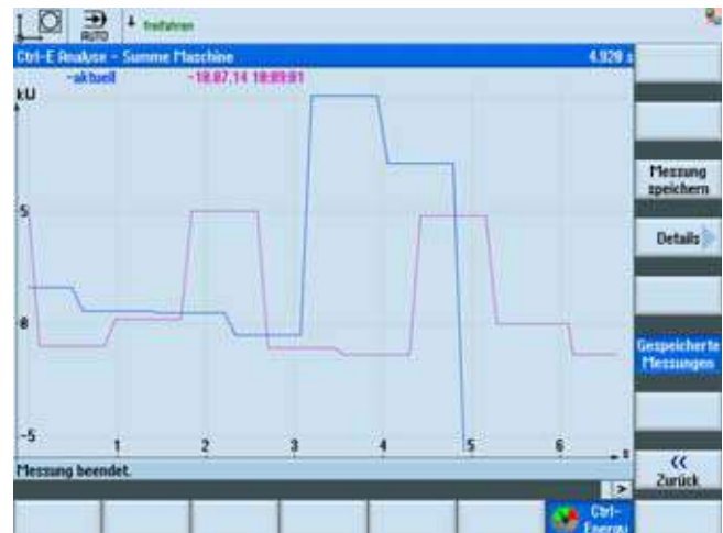
Graphical comparison of two measurements for qualitative evaluation of a machine tool's energy consumption
