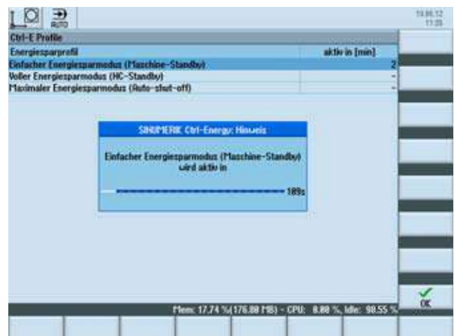
Overview of defined energy-saving profiles for a machine tool – with pre-alarm window in the foreground
