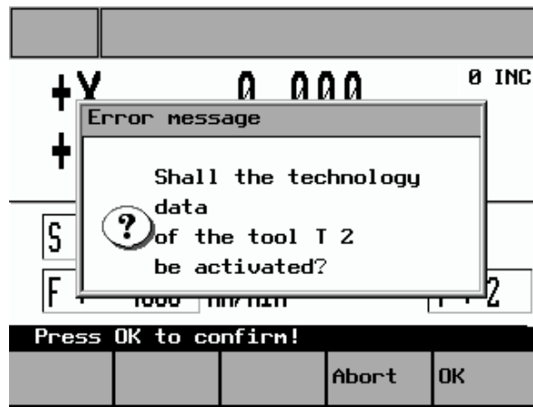
Fig. 2-6: Tool technology data acceptance message
