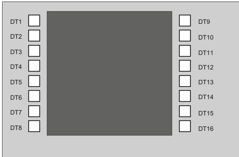
Image 1-7 Assignment of the direct keys to the vertical softkeys of an operator panel front
