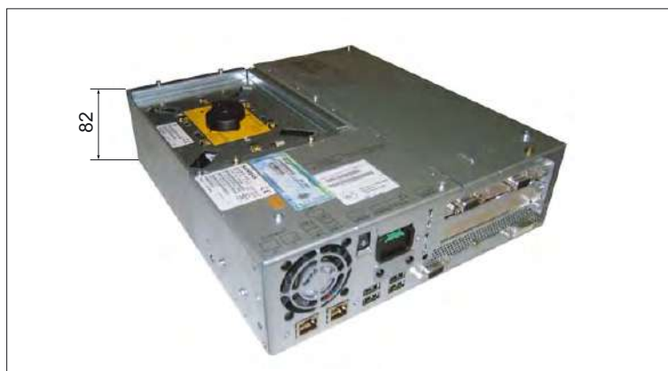
Figure 19-1 Perspective view of PCU 50.3 (without plug-in card)
