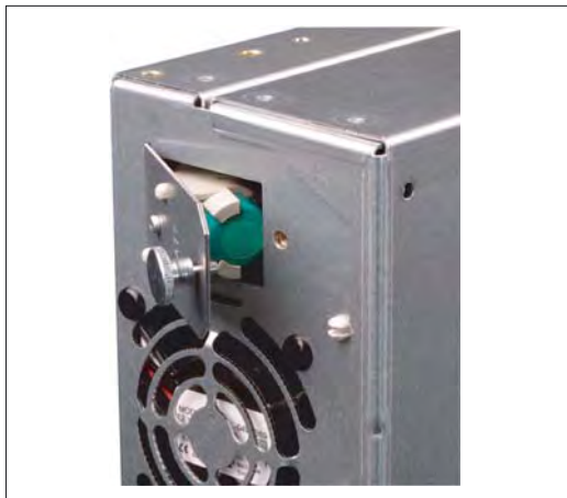
Figure 19-29 Opening the battery compartment
