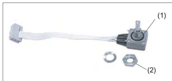
Figure 23-19 Dismantled rotary override switch
