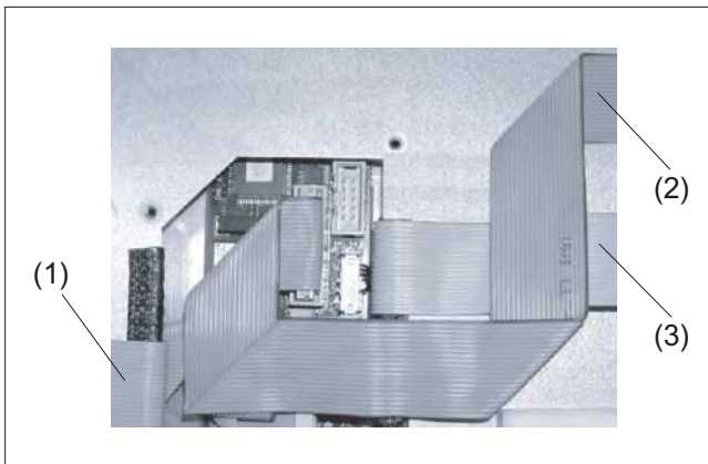
Figure 16-17 TP 015A: DKM cable routing
