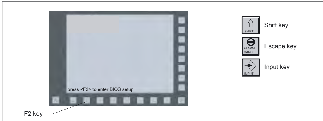
Figure 18-9 PCU 50: Using the BIOS Setup via an operator panel front
