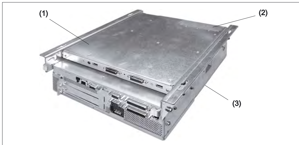
Figure 21-13 PCU/transmitter unit assembled for "flat" mounting
