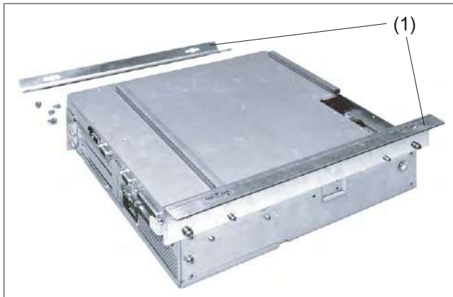
Figure 14-15 PCU 50 with mounting brackets
