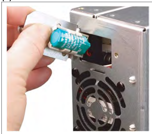
Figure 19-30 Removing the battery holder
