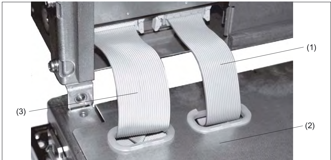
Figure 8-2 Connections on rear side of housing Connections to the PCU
