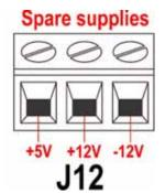
An appropriate voltage supply is available where required on each connector. In addition, supplies may be drawn from the Spare supplies connector (J12).
