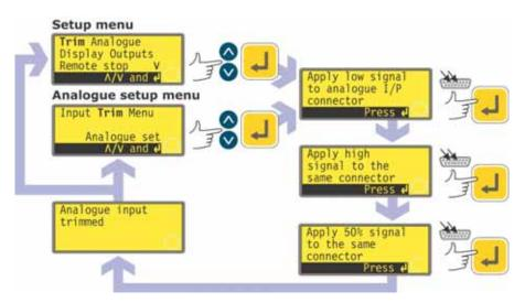
When the pump is under remote control, it tracks an analogue signal from the user's remote control system to the **i/p** terminal of the Analogue 1 connectors at the rear of the pump within the ranges 4-20mA, 0-10V or 1-5V. The **Trim** setup sequence allows the user to customise the process-signal-to-pump-speed calibration. The sequence may be entered directly from the Setup menu or from the Analogue setup menu.
