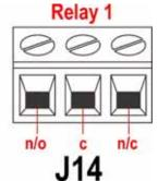
to indicate General alarm status. See 12 Switching the pump on for the first time.
