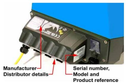
The same information is carried on the drive's backplate, accessible when the 720N module is removed. The number of connectors varies according to the model.
