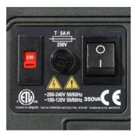
**Input line fusing**: type T5A H 250V 20mm time-delayed cartridge fuse, located in a fuseholder in the centre of the switchplate at the rear of the pump.
