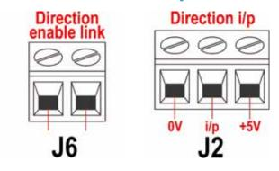
To enable remote direction control and disable the **DIRECTION** (**SHIFT**, **1**) key on the keypad, link the terminals of the Direction enable link connector (J6). **Important: Apply no voltage whatever to the Direction enable link.** Connect a remote switch between the **+5V** terminal and the **i/p** terminal of the Direction i/p connector (J2). Open switch for
