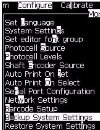
Figure 4-37: Backup System Settings
