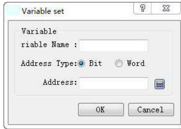
Figure 7-16 Create a screen switch through bit control dialog box
