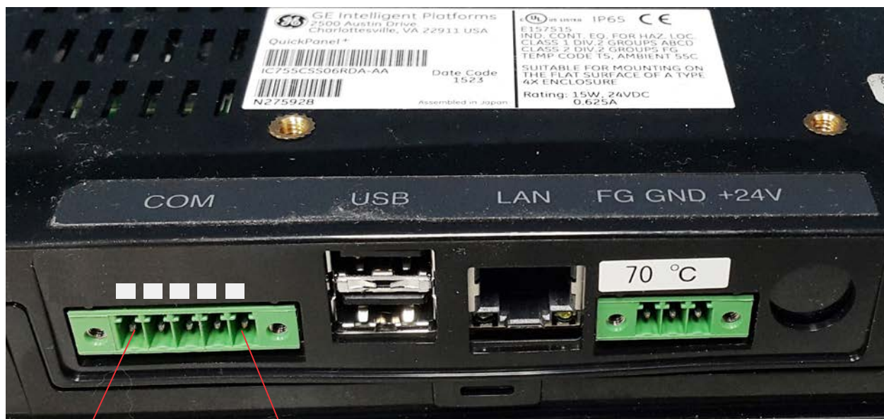
IC755CxS06RDx Serial Port COM1 Pin-out
