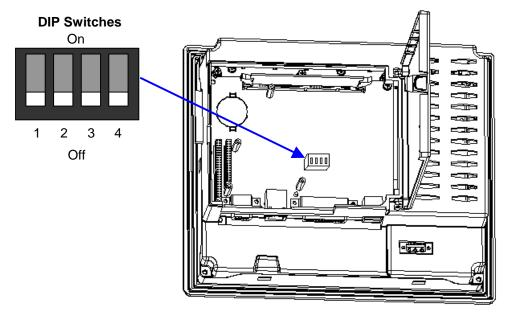
When the switch is set to "OFF", the QuickPanel View/Control operates normally, displaying the startup splash screen. You can skip running the startup applications by tapping the "Don't run StartUp Programs" button on the startup splash screen.
