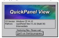
When the switch is set to "ON", the startup programs are forced to run and the "Don't run Startup Programs" button is not available on the startup splash screen.
