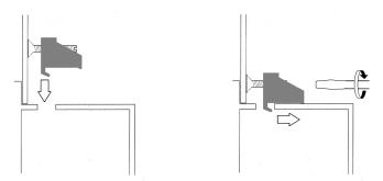
Do not damage the gasket attached to the back of the QuickPanel View Keypad's bezel. This gasket prevents shock hazards and damage caused by liquids accidentally entering the unit after installation.
