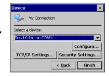
6. From the list, choose the device or modem you want to use. (If a Modem or Serial CF Card is inserted, it will be available in the device list.)
