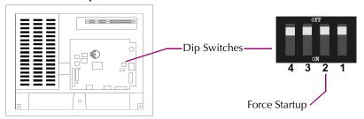
When the switch is set to "OFF", the QuickPanel View Keypad operates normally, displaying the startup splash screen. You can skip running the startup applications by tapping the "Don't run StartUp Programs" button on the startup splash screen.
