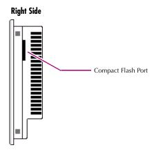
A CF card is inserted in this port with the card's front facing the back of the unit (the narrow side slot on the card should be toward the bottom).
