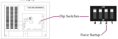
When the switch is set to "OFF", the QuickPanel View/Control operates normally, displaying the startup splash screen. You can skip running the startup applications by tapping the "Don't run StartUp Programs" button on the startup splash screen.
