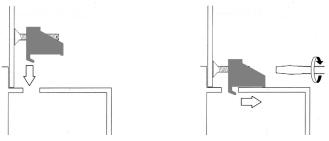
Do not damage the gasket attached to the back of the QuickPanel View/Control's bezel. This gasket prevents shock hazards and damage caused by liquids accidentally entering the unit after installation.
