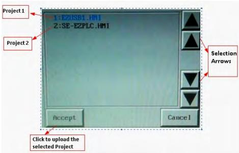
Select the required project using the Up-Down arrows and press "Accept." If the panel is not compatible with the project selected, an Error message saying "Wrong panel Type" is displayed. The selected project is then automatically loaded into the EZTouchPLC.
