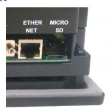
A Micro SD slot is available for data logging purposes. Additional details about using a MicroSD Card for data logging is available in the *Data Logging Overview* section. Push against the Micro SD card to eject it from the Touch I/O unit when finished.
