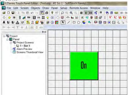
4. Similarly, you can create an Indicator Light Object by selecting **Objects > Data Display > Indicator Light**. Enter **Lamp** for Tag Name. Click OK. Place the object on the panel. Your screen should look like the picture below.
