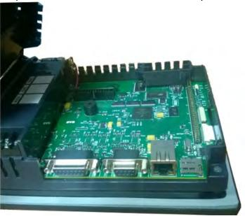
2. The battery is located in the upper-left hand corner as shown in the figure below. Remove the old battery and replace with a new 1/2 AA, 3.6 V Lithium Battery (Part Number: **EZ-BAT**).
