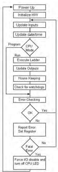
A good understanding of the EZTouchPLC CPU operating sequence will help you achieve the proper control for your equipment or process. The flow chart on the left shows how the CPU controls all aspects of system operation.
