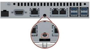
Be sure to hit the button accurately and do not slide the tool off the button.
