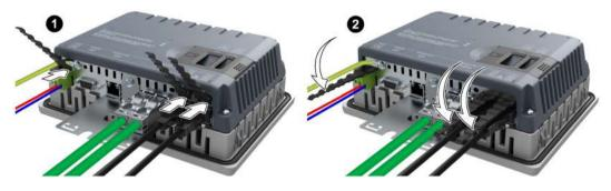
Next, use cable ties to secure the cables to the marked fixing elements.
