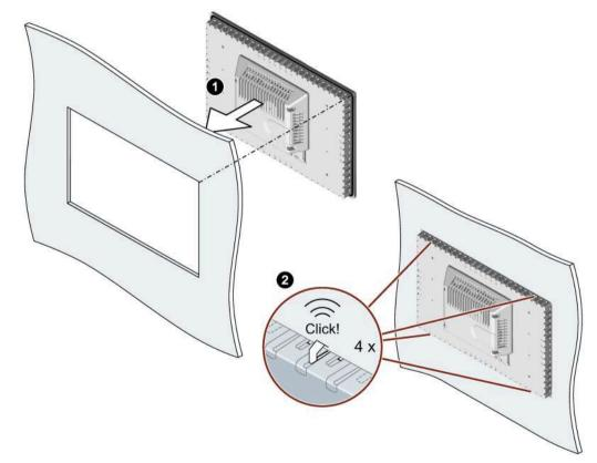
2. Make sure that all four spring locks on the top and bottom of the device fully engage. If necessary, gently press the device into the recess if it is not fully engaged.
